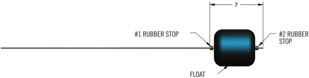
3. Insert the float rod into the stand-off hole. Slide on rubber stop (#3) 8" from the top of the rod. Slide the float rod through the hole in the lever. Then slide on rubber stop (#4) 1" above rubber stop (#3).
