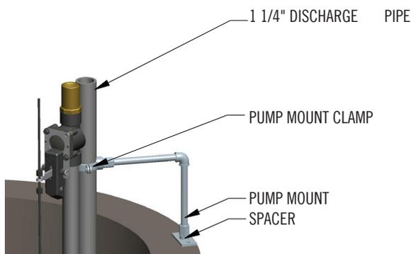
The float rod must easily move up and down and be in the vertical position. Make sure the float does not interfere with the electric sump pump, power cord or side of the basin.
